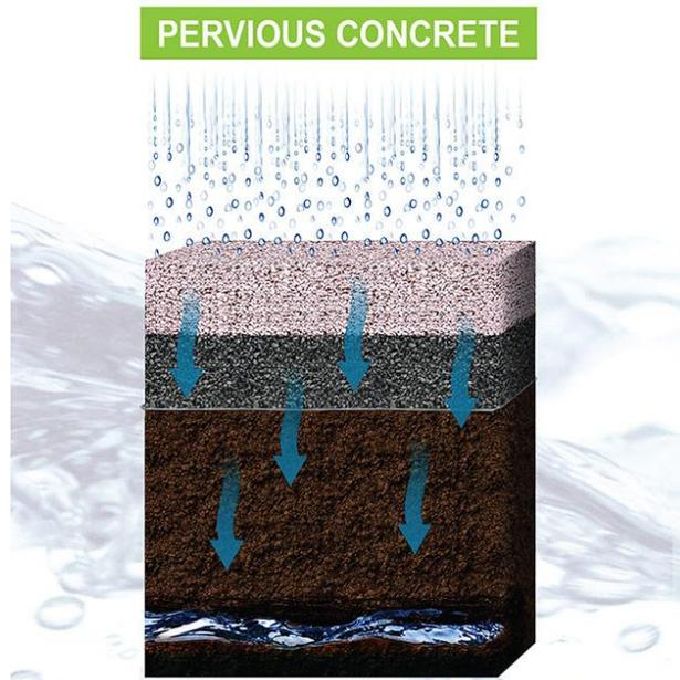
c. Permeable concrete does require some maintenance to retain its permeability.
